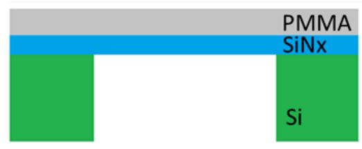
Figure 1. A not-to-scale schematic of a membrane. The silicon nitride layer is commonly 50 – 200 nm thick, and the silicon frame is commonly 0.2 – 7 mm.
